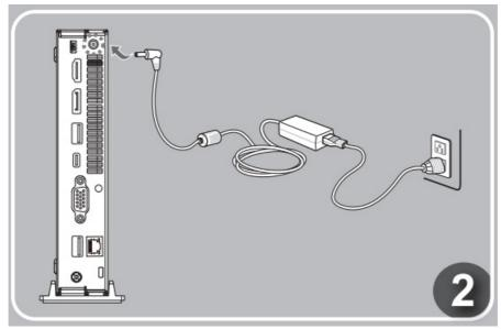
2. Connect the power cord to the system and electrical outfet,
