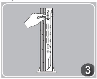
3. Press the power button to power on the system,
