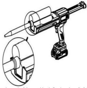
4.2 Insert the cartridge. Make sure the neck of the cartridge is fixed on the rail of the holder.
