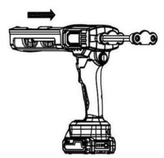
4.1 Press the clutch plate and pull backward the rod.
