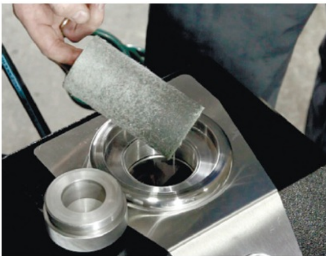
Fig. 6. Filter element after the first flushing cycle.
