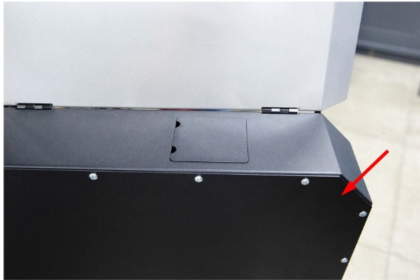
Figure 1. Dismountable panel of the bench enclosure
