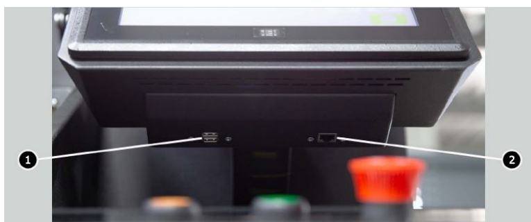
Figure 4. Position of USB and LAN ports
