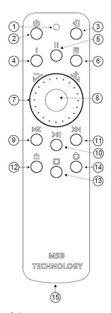
When changing settings in the menu, use the enter button in the center of your volume wheel on the remote or the right arrow on the DAC faceplate to confirm settings in the DAC menu. After you have made your changes in the DAC menu, use the menu button to exit the DAC menu completely to save the changes you have made in the DAC menu.
