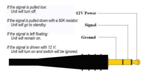
12 Volt Remote Trigger wiring.
