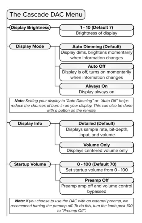
**Note**: If you choose to use the DAC with an external preamp, we recommend turning the preamp off. To do this, turn the knob past 100 to "Preamp Off".
