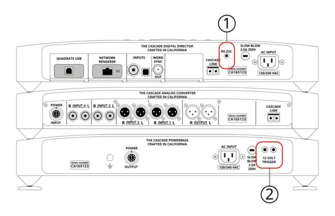
**RS-232:** The Digital Director features an RS-232 control port on the back of the unit that can be used with whole home control systems and for home theater integration. A full list of commands and coding can be found using the QR code below.
