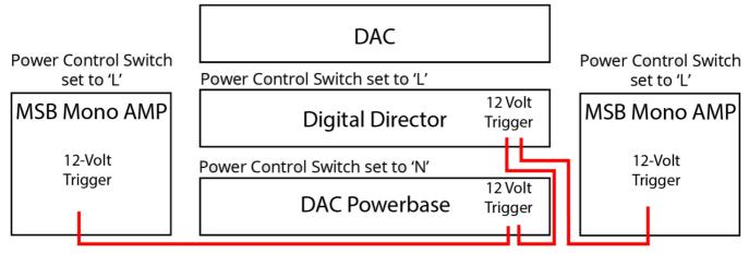
The diagram above is only a visual example and the actual connections may vary in your system. The specific order in which the units are connected does not affect how the 12 volt connections will function. The only requirements are that each unit is connected to a 12 volt trigger port of another unit in the chain. Only one unit is set to the normal `N' position while all other units are set to the linked `L' position.
