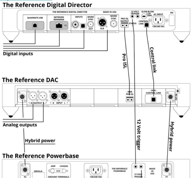
When installed properly, your system should look like the example above. The digital inputs installed in your digital director may vary depending on what sources are in your system, However; the only modules that should be installed in the DAC will be the provided Pro ISL and Control Link modules as well as any analog input modules you may have in your system.
