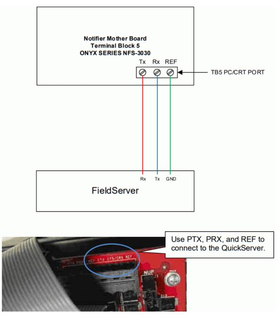
The printer port must be enabled on the unit and set to 80 columns with NO supervision unless port supervision is enabled in the driver configuration.
