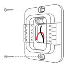
4. Step 4: Smart Wi-Fi Mini-Stat has two terminals marked as Rc and C on its backplate. Insert red wire into Rc and black wire into C from the side (press the terminal block buttons for ease of insertion).
