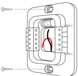
**Step 4:** Smart Wi-Fi Mini-Stat has two terminals marked as Rc and C on its backplate. Insert red wire into Rc and black wire into C from the side (press the terminal block buttons for ease of insertion).
