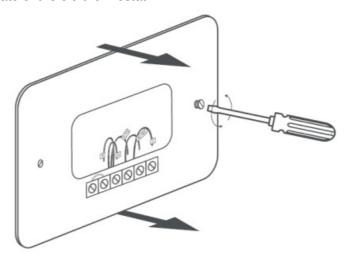
• Step 7: Optional-You may use the provided wall plate to hide any marks or holes on the wall left by the old thermostat installation.
