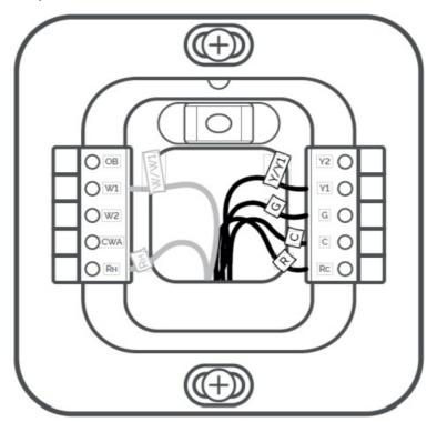
• Step 11: Gently push the excess wires back into the wall hole to ensure that no drafts are coming from it.
