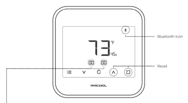
First, check that the **thermostat set points are 00**. If not, press and hold the **Temperature Up** and **Presets** buttons simultaneously until all the buttons vanish. The **Bluetooth** icon will start blinking, and you can begin the registration process.
