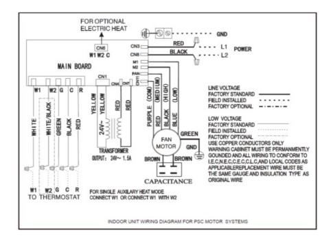
Note: Description of Fan Speed Switch with PSC Motor
