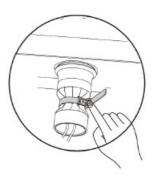
2. After installation or maintenance, the tightening belt shall be tightened, and should not be loosened or
