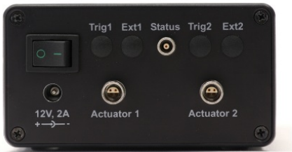
Figure 6: Power input and output connectors on left side
