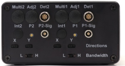
Figure 7: Input connectors, P factor adjustment and switches on right side
