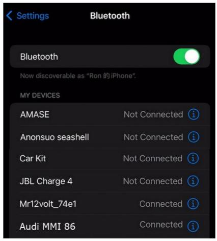
• Mr12volt Does not support the integration of OEM microphone even with the installation of a Y-cable. if you need to use Mr12volt HF or Voice Command such as SIRI, the 3.5mm jack microphone supplied in the package must be installed.
