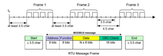
The entire message frame must be transmitted as a continuous stream of characters. If a silent interval of more than 1.5 character times occurs between two characters, the message frame is declared incomplete and should be discarded by the receiver.
