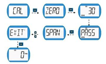
Or, using the short-cut Zero button on the remote programmer:
