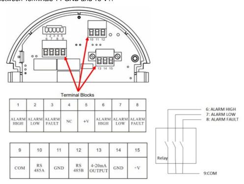
Alarm outputs on Terminals 6-9 are normally-open dry contacts that close on alarm. The 4-20 mA output should be connected to Terminals 13 and 14. RS485 should be connected to terminals 10 & 12, and terminal 11 is for the RS485 shielding line. The +V terminals 5 and 15 are equivalent and internally connected, as are GND terminals 11 and 14.
