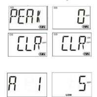
From the EVT LOG screen, long-press until the beep toshow the latest alarm event A1 and then short-pressrepeatedly to cycle through the last 10 alarm events lasting≥5 seconds. Up to 50 alarm events are logged into memory.
