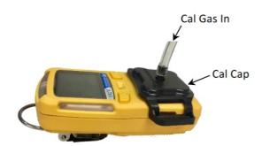
Press Left [+/OK] again. A 10-second count-down starts. When finished, "Pass" or "Fail" displays. To abort, Press Right  $[^{\bullet}/\downarrow]$  at any time during the count-down.
