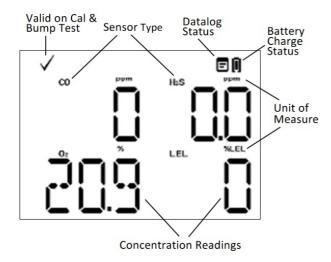
Press Right  $[^{0}/_{\downarrow}]$  to scroll through the main menu and view the maximum values, minimum values, STEL, TWA, date, time, LEL measurement gas and correction factor, and LEL calibration gas.
