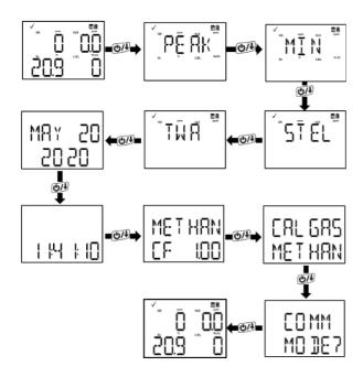
From the last screen "Comm Mode", press the Left [+/OK] key to enter PC communication mode to download data and upload configurations.
