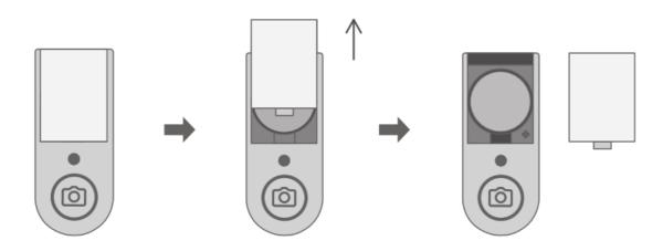
When the power is low due to long-term use, tightly push the battery cover of the upper part of the remote control upward to replace the new button battery.
