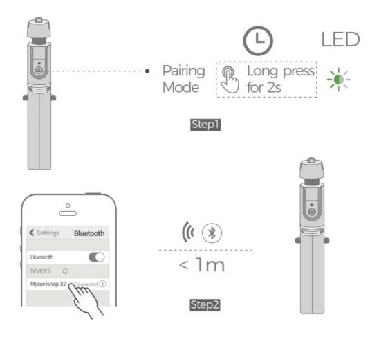
Long press the camera key for 2s until the green light flashes. Turn on the wireless function on your phone and select "Mpow isnap X2", the green light off if paired successfully.
