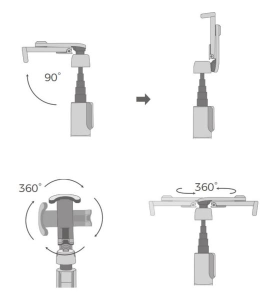
4 Unfold and Fix the Tripod
