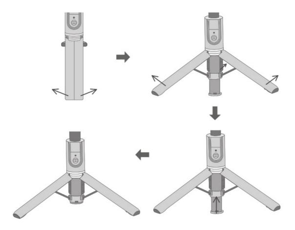
Unfold the tripod and push the center column upward until the tripod is fully expanded and stable. Place it on the flat surface to take photos.
