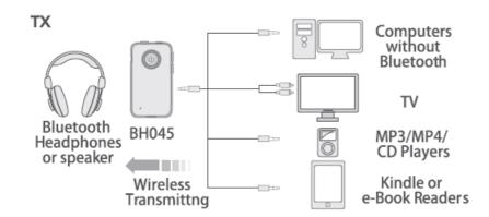
Connect BH045 to a Non-Bluetooth multimedia audio device (such as 1V. PC) with a 35 mm audio cable. RCA cable. Then, pair BH045 to a Bluetooth headphone/ Bluetooth speaker. In this way, BH045 can transmit music from a Non-Bluetooth multimedia audio device (such as 1V, PC) to a Bluetooth headphone/ Bluetooth speaker
