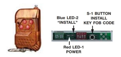
Installing the Key FOB: Matching the Key FOB (Clicker) to the Receiver NOTE: Units are "Pre-Matched" at the factory.
