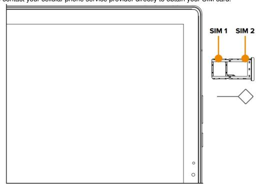
To insert SIM card(s): Eject the SIM/SD card holder using the SIM removal tool.
