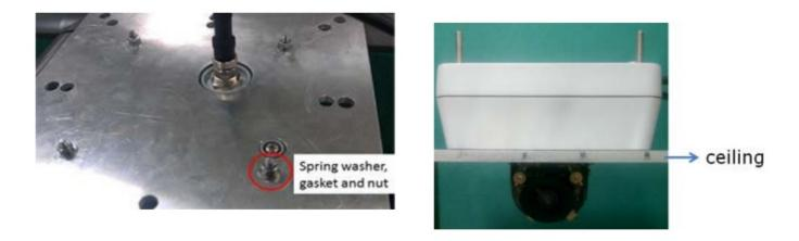
Step 5: Loosen the screws that fix the horizontal and vertical lens positions. Next, tune the camera lens position, and connect to the VPort P16's web console to view the video image. After the lens position is correct, fix the screws (5.5 kgf-cm torque is required).
