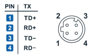
**NOTE** To connect the VPort P16-2MR series to the network, use an Ethernet cable with a D-code M12 connector and an M12 PoE switch or RJ45 PoE switch
