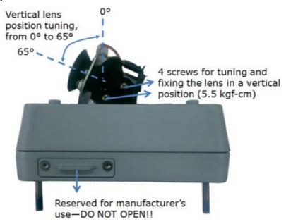
4 screws for tuning and fixing the vertical lens position: There are 4 screws for tuning and fixing the vertical lens position. The vertical lens position can be tuned from 0° to 65°. A 5.5 kgf-cm torque is required for onboard environments
