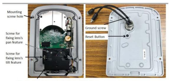
Calibration for tuning lens's vertical (-5 to 10  $^\circ$  )and horizontal (+/- 5  $^\circ$  ) position
