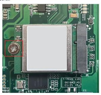
2. Fasten the silver screw to secure the module.
