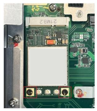
2. Fasten two black screws to secure the module.
