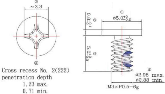
Use 2 screws (M3\*5L standard is recommended) on each side to attach the V3200 to a wall or cabinet. These 4 screws are not included in the product package; they need to be purchased separately. Ensure that the V3200 computer is installed in the direction shown in the following figure:
