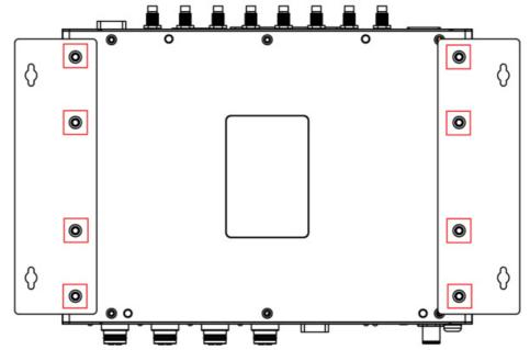
The 8 screws for the mounting brackets are included in the product package. They are standard IMS\_M3x5L screws and require a torque of 4.5 kgf-cm. Refer to the following illustration for details.
