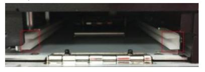
6. Insert the tray so that it aligns with the rails on both sides and slide the tray into the slot.
