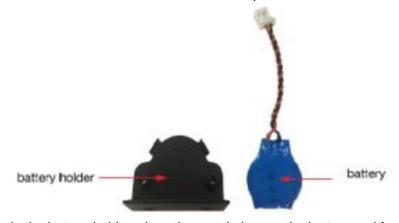
5. Replace the new battery in the battery holder, place the metal plate on the battery and fasten the two screws tightly.
