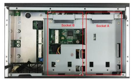
6. To place the storage disk tray, put the end of the tray near the groove on the socket.
