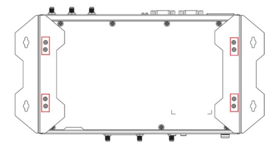
The eight screws for the mounting brackets are included in the product package. They are standard IMS\_M3x5L screws and require a torque of 4.5 kg-cm. Refer to the following illustration for details.
