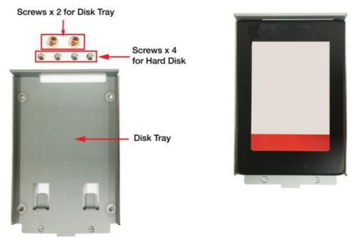
3. Turn the disk and tray arrangement around to view the rear side of the tray. Fasten the four screws to secure the disk to the tray.
