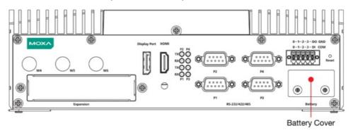
2. Unfasten the two screws on the battery cover.
