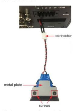
4. Separate the connector and remove the two screws on the metal plate.
