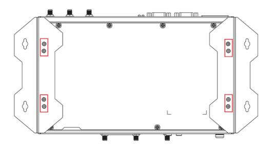
The eight screws for the mounting brackets are included in the product package. They are standard IMS\_M3x5L screws and require a torque of 4.5 kgf-cm. Refer to the following illustration for details.
