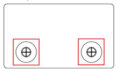
3. Take off the cover; the battery is attached to the cover.
