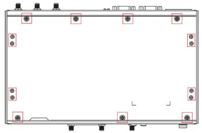
5. Take out the rear cover of the computer and find the location of the storage disk sockets. There are two sockets for the storage disk tray; you may install on either socket.
