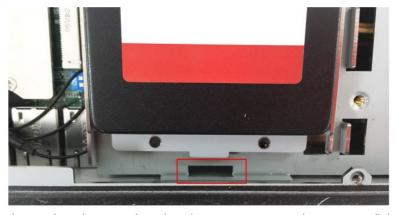
7. Place the tray on the socket and push upward so that the connectors on the storage disk tray and the socket can be connected. Fasten two screws on the bottom of the tray.
