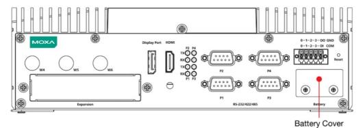
2. Unfasten the two screws on the battery cover.
