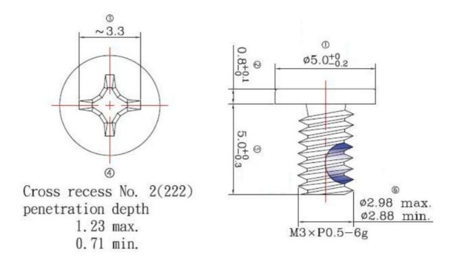
Use two screws (M3\*5L standard is recommended) on each side to attach the V2403C to a wall or cabinet. The product package does not include the four screws required for attaching the wall-mounting kit to the wall; they need to be purchased separately. Ensure that the V2403C computer is installed in the direction shown in the following figure.
