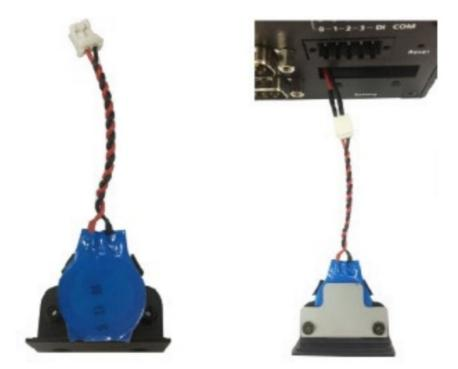
6. Reconnect the connector, place the battery holder into the slot, and secure the cover of the slot by fastening the two screws on the cover
