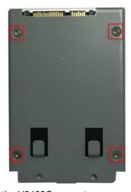
4. Remove all screws on the rear panel of the V2403C computer.
