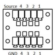
The V2201 comes with 4 digital inputs and 4 digital outputs on a 2×5 terminal block.
