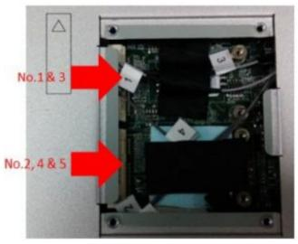
5 connectors are attached to the mini-PCle sockets:
