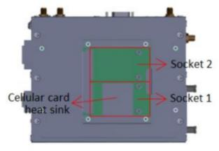
NOTE: The cellular card heat sink is installed in socket 1.
