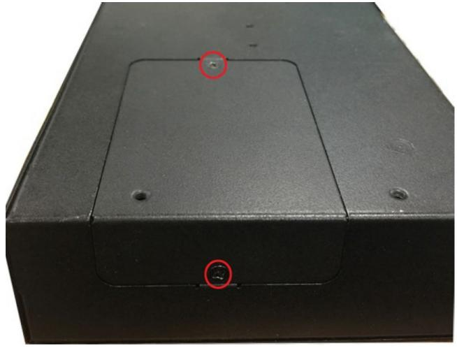
2. Remove the cover to access the SD-card slot and the mSATA
