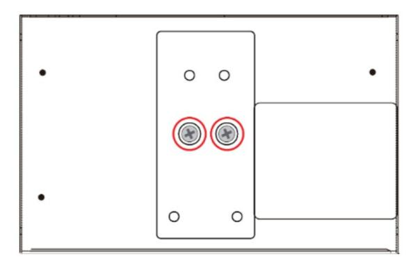
Use another four screws to fasten the DIN-rail mounting plate.
