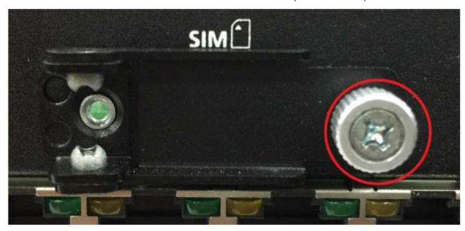
2. Insert the SIM card into the slot. Make sure you insert the card in the direction indicated above the card slot.
