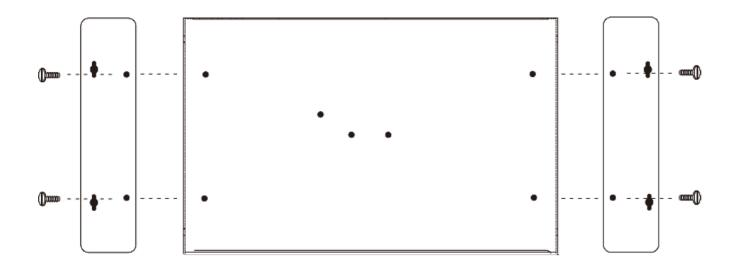
These four screws are included in the wall-mounting kit. Refer to the right figure for the detailed specifications.
