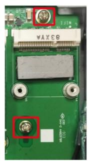
3. Install the Wi-Fi module in the socket and fasten two black screws on the module. Also, fasten the two bronze screws on the board.
