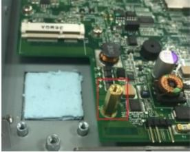
10. Attach one thermal pad to the cellular module cover and the other thermal pad to the module pad.
