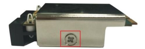
13. Insert the module into the socket and secure it using a screw from the package.
