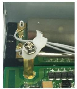
18. Plug the antenna onto the connector.
