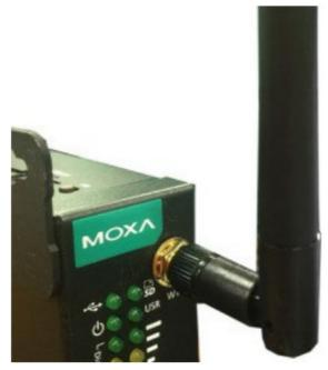
There are three antenna connectors on the front panel of the UC-8100A-ME-T. W1 and W3 are for cellular modules, and W2 is for the GPS module. All three connectors are of SMA type.
