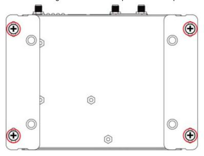
**Step 2**Use another four screws to mount the computer on a wall or a cabinet.
