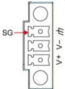
**SG:** The Shielded Ground (sometimes called Protected Ground) contact is the top contact of the 3-pin power terminal block connector when viewed from the angle shown here. Connect the SG wire to an appropriate grounded metal surface.
