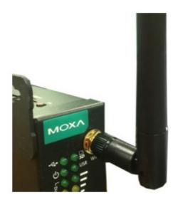
There are three antenna connectors on the front panel of the UC-8100A-ME-T. W1 and W3 are for cellular modules, and W2 is for the GPS module. All three connectors are of SMA type.
