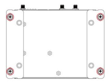
**Step 2**Use another four screws to mount the computer on a wall or a cabinet
