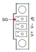
**SG:** The shielded ground (sometimes called protected ground) contact is the top contact of the 3-pin power terminal block connector when viewed from the angle shown here. Connect the SG wire to an appropriate grounded metal surface.
