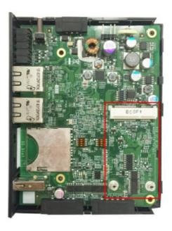
3. Remove the plastic plate and the sticker on both sides of the **large** thermal pad and place it in the socket. Press the thermal pad down so that it sticks to the base of the socket. Place the thermal pad as close as possible to the holes for the screws used to secure the module.
