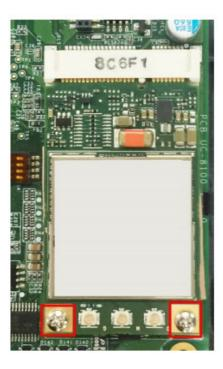
5. Remove the plastic plate and the sticker on both sides of the **small** thermal pad and stick the thermal pad onto the module.
