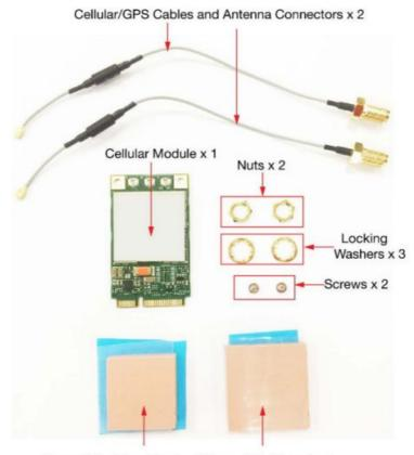
Thermal Pad (small) x 1 Thermal Pad (large) x 1
