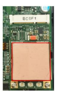
6. Install the antenna cables. There are three antenna connectors on the module; two for cellular antennas and one for a GPS antenna. Refer to the figure for details. As there are only two antenna connector holes on the front panel of the computer, you can only use two antennas at a time. You may use two cellular antennas, or a cellular antenna and a GPS antenna. The same antenna cables can be used for both antenna types.
