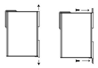
Another method for wall mounting installation is to use the optional wall mounting kit. Attach two mounting brackets on the side panel of the computer, and fasten them with screws. Install the computer onto a wall or cabinet by fastening two screws for each mounting bracket.
