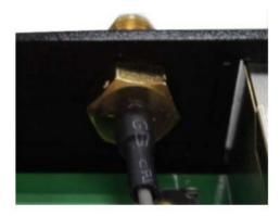
9. Insert the locking washer through the connector and press it against the cover of the computer. Then, insert the nut and tighten it to secure the connector to the cover.
