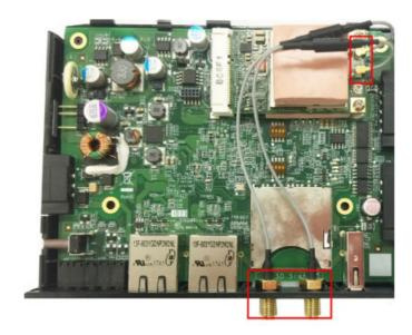
8. Insert the other end of the cable, with the connector, through the antenna connector hole on the front panel of the computer. Remove the black plastic protective cover on the connector hole before you insert the antenna wire.
