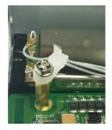
18. Plug the antenna onto the connector.
