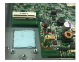
10. Attach one thermal pad to the cellular module cover and the other thermal pad to the module pad.
