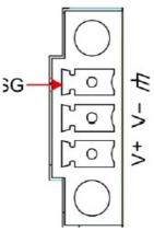
**SG:** The Shielded Ground (sometimes called Protected Ground) contact is the bottom contact of the 3-pin power terminal block connector when viewed from the angle shown here. Connect the SG wire to an appropriate grounded metal surface.
