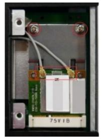
5. Connect the antenna adapters to the connectors on the front panel of the computer.
