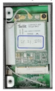
2. Connect the free ends of the two antenna cables to the RX diversity antenna (labeled D) and the main RF antenna (labeled M) as shown in the figure.
