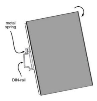
**Step 2:** Push the UC-5100 towards the DIN rail until the DIN-rail attachment bracket snaps into place.
