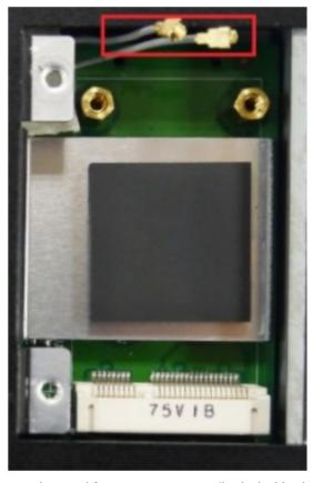
2. Insert the cellular module into the socket and fasten two screws (included in the package) on to the top of the
