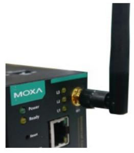
Connect the cellular antennas to the connectors.
