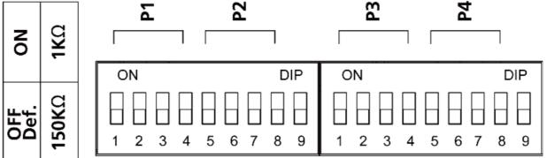
Each port consists of 4 pins; you must switch all 4 pins of a port simultaneously to adjust the value of the port.
