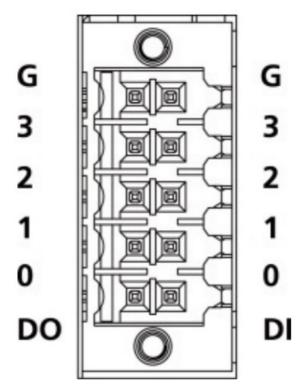
The UC-5100 Series computer comes with 4 general-purpose input connectors and 4 general-purpose output connectors. These connectors are located on the top panel of the computer. Refer to the diagram on the left for the pin definitions of the connectors. For the wiring method, refer to the following figures.
