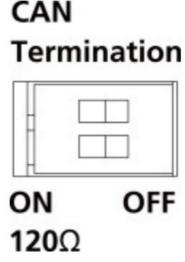
2. Adjust the setting as required. The ON value is  $120\Omega$ , and the default value is OFF.
