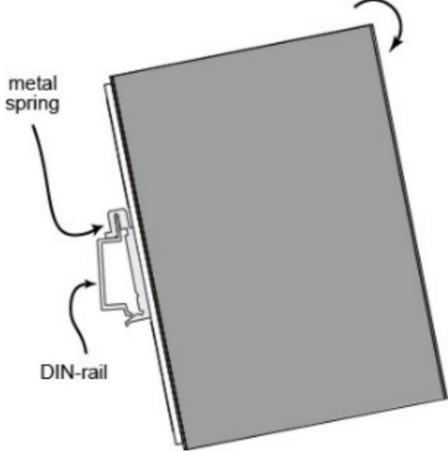
**Step 2**Push the UC-5100 towards the DIN rail until the DIN-rail attachment bracket snaps into place.
