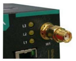
5. Connect the antenna adapters to the connectors on the front panel of the computer.
