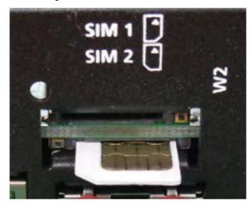
To remove the Micro SIM card, simply push the Micro SIM card and release it.
