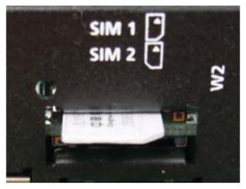
Insert the Micro SIM card into the socket.Make sure you place the card in the right direction.
