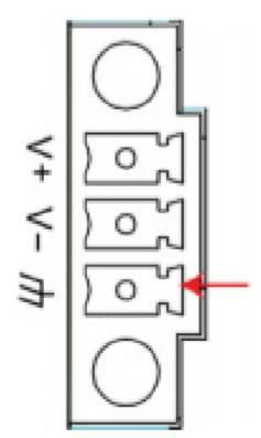
**SG:** The Shielded Ground (sometimes called Protected Ground) contact is the contact at the bottom of the 3-pin power terminal block connector when viewed from the angle shown here. Connect the wire to an appropriate grounded metal surface or to the grounding screw on top of the device.
