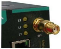
6. Connect the Wi-Fi antennas to the antenna adapters.
