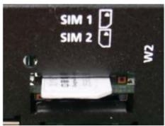
2. Insert the Micro SIM card into the socket. Make sure you place the card in the right direction. To remove the Micro SIM card, simply push the Micro SIM card and release it.
