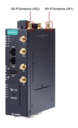
• In addition, a GPS antenna connector is provided for the GPS module. All cellular and GPS connectors are of type SMA female.
