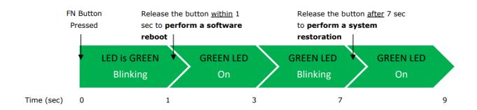
The mapping of the action on the FN button with the behavior of the SYS LED and the resulting system status is given below:
