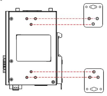
2. Use two screws to mount the UC-3100 onto a wall.
