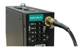
There are three antenna connectors on the front panel of the UC-2200A. W1 and W2 are for cellular modules. A GPS antenna connector is located at the top of the front panel. All three connectors are of SMA type.
