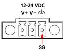
SG: The Shielded Ground (sometimes called Protected Ground) contact is the right-most contact of the 3-pin power terminal block connector when viewed from the angle shown here. Connect the SG wire to an appropriate grounded metal surface.
