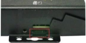
To remove the MicroSD card, simply push the card in and release it.
