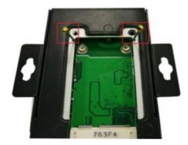
2. Insert the cellular module into the socket and fasten two screws (in the package) on to the top of the module
