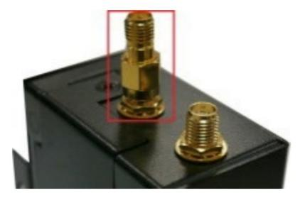
6. Connect the Wi-Fi antennas to the antenna adapters.
