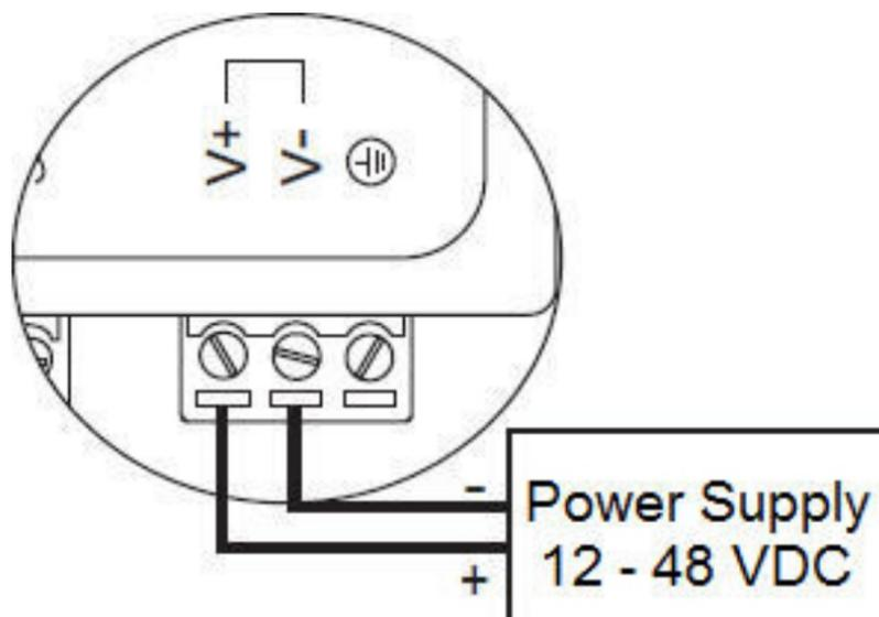
The TCC-100 is powered by an external 12 to 48 VDC power supply. To connect the power supply, run two wires from the V+ and V- terminals on the TCC's 3-conductor terminal block to the DC power supply, as shown in the figure. Once the power supply is connected to its power source, the PWR LED located on the TCC's top panel should turn red.
