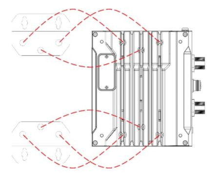
**STEP 2:** Mounting the TAP-M310R Series to a wall requires 4 screws. Use the device with the wall-mounting plates attached as a guide to mark the location of the 4 screws on the wall. The heads of the screws should be between 5.5 mm and 8.5 mm in diameter. The screw shank should be between 2.4 to 3.98 mm in diameter. The screw length should be at least 15.0 mm, as shown in the figure on the right.
