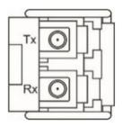
**NOTE** 1000/2500BaseSFP ports that are not in use should be covered with an IP67-rated plastic cap.
