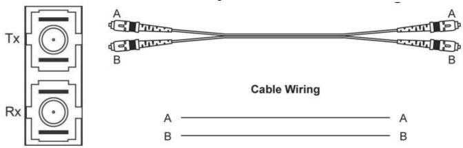
ST-Port Pinouts ST-Port to ST-Port Cable Wiring
