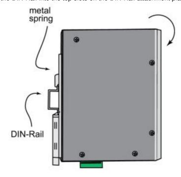
**STEP 3:** The DIN-Rail attachment unit will snap into place as shown in the following illustration.
