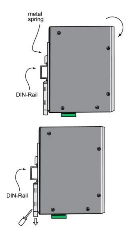
To remove the Moxa PT-508 switch from the DIN-Rail, use a screwdriver to push down the spring-loaded bracket until it locks in place, as shown in the following diagram. Next, rotate the bottom of the switch upwards and then remove the switch from the DIN-Rail.
