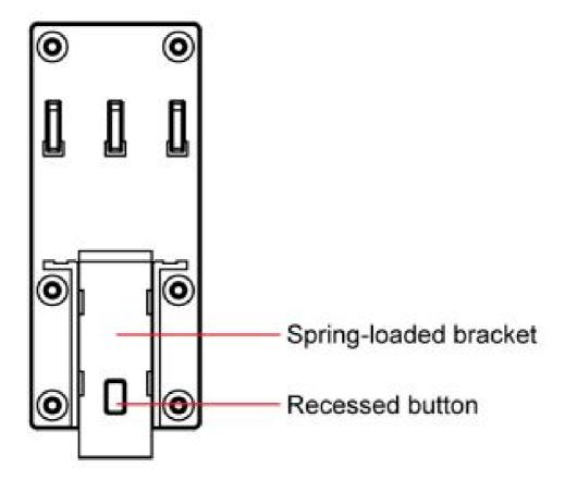
**STEP 2:** Insert the top of the DIN-Rail into the top slots on the DIN-Rail attachment plate.
