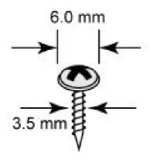
**NOTE** Test the screw's head and shank size by inserting the screw into one of the keyhole-shaped apertures of the wall mounting plates before screwing it into the wall.
