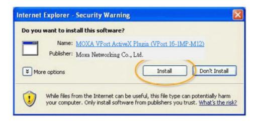
**NOTE** For Windows XP SP2 or above operating systems, the ActiveX Control component will be blocked for system security reasons. In this case, the VPort's security warning message window may not appear. Users should unlock the ActiveX control blocked function or disable the security configuration to enable the installation of the VPort's ActiveX Control component.
