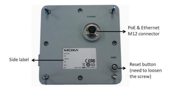
• PoE & Etherent M12 connector: A 4-pin M12 D-code connecter for both PoE power supply (Mode A) and Auto MDI/MDI-X Ethernet connection.
